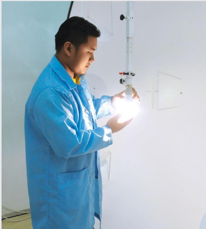
*A lab technician at the photometry test facility placing a bulb into the integrating sphere which measures the light characteristics of lamps.*
